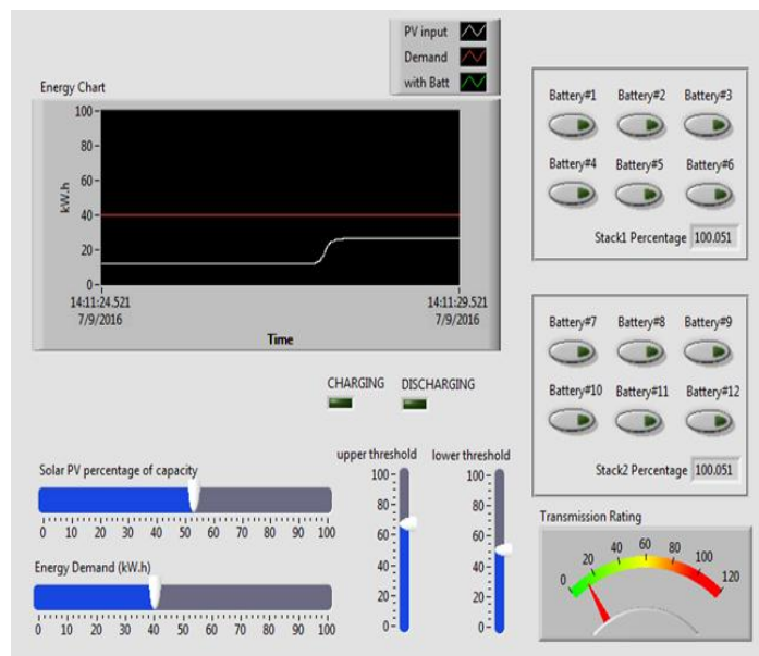
Figure 2. Labview graphic interface of hybrid energy storage
