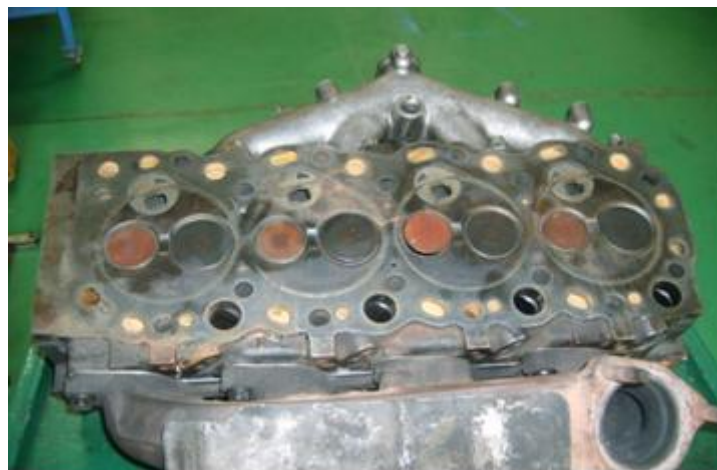
Figure 1. shows the cylinder head and the modified wood burn chamber position
