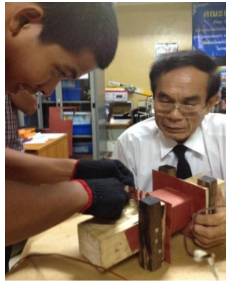
a) Arrangement the hard fiber form to support all the coil windings
