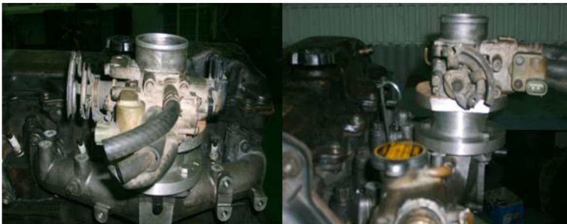
Figure 3. Installs Thottle valve
